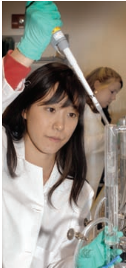
Research assistant Jennifer Huang delivers nutrient solution containing glucose to a tissue bathing solution. Tissues mounted on Ussing chambers can be kept healthy for as long as six hours.
