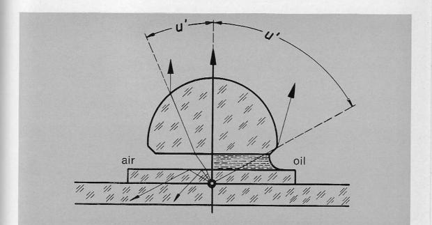
Fig. 31 shows the gain in aperture by oil immersion (right) as compared with a dry objective (left) What is the resolving limit?
