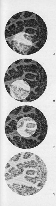
1. Align microscope illuminator with plane mirror of the microscope and adjust it so that a small, bright spot of light is projected onto the mirror or an image of the filament formed (this adjustment is facilitated if a sheet of paper is held over the surface of the mirror).
