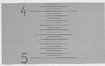
Fig. 39 Eyepiece micrometers
