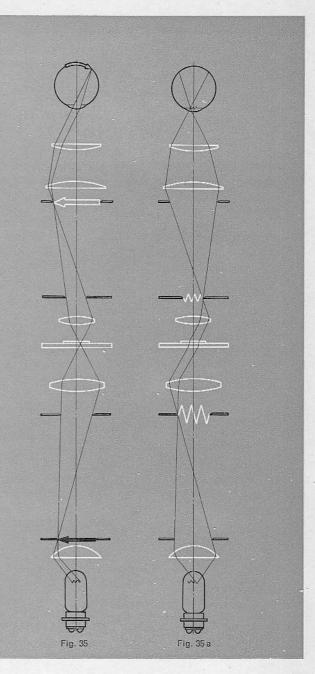
4. Viewed from the specimen, the light source is at infinity (parallel rays in the aperture ray path, Fig. 35a). Any irregularity in the source is therefore least effective in the specimen plane.
