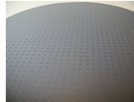
Figure 8: Image of an array of micro-lenses (diameter of lenses: 1 mm, height of lenses: 500 μm) imprinted with working stamp on 200 mm glass wafers
